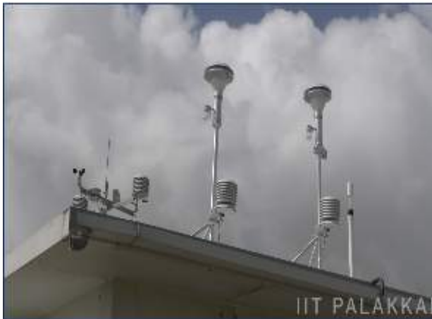
Air quality measurement station
