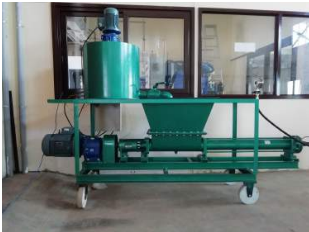
Grout Pump for Field Tests
